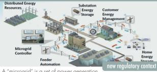
A "microgrid" is a set of power generation, storage, and transmission facilities that can connect and disconnect from the larger grid, creating a more resilient energy system and one in which local control can be exercised over the entire circuit of policy support energy creation, purchasing, sale, and utilization.
